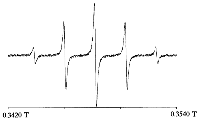
Figure 2. A multiple-line spectrum typical of coupling of the unpaired electron to four equivalent protons as in the alanine radical, \text{CH}_3\text{CH}_2\text{COOH} . Nominal frequency: 9.765 GHz.
