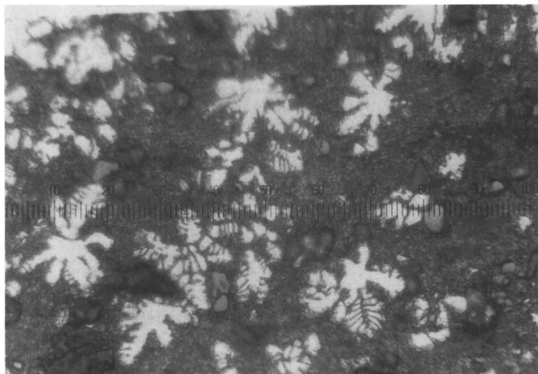
Figure 13. Copper dendrites inside a large particle of lead in coin A-271. The length of the smallest division on the scale is 2.5 \mu\text{m} .
