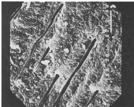
Figure 3. SEM photomicrograph of same bone as Figure 2 cut parallel to blood vessels (dark areas). The thin bright area along the edge of the voids left by the blood vessels are calcium sulfate (gypsum or anhydrite).
